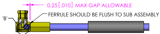
IN-PROCESS 4 CRIMP FERRULE (USE RF CRIMP HAND TOOL #CAT-RF-FER-01, AND .128" DIE SIZE)
