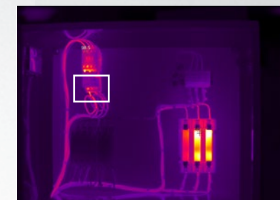
Full image, taken from 5 feet away with a TiX1000 infrared camera. The area shown in the white box is blown up below.
