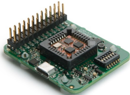
Figure 1: MTi 1-series Development Board with MTi-3-8A7G6 module
