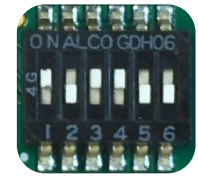
Figure 7: Switch to I 2 C interface and VDDIO of 3.0V
