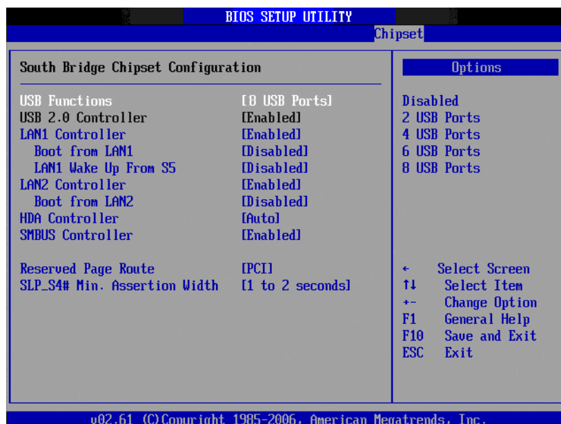
Figure 3.13 South Bridge Configuration
