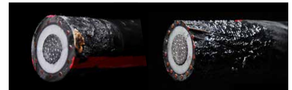
Cable Protected with Scotch® Fire Retardant Electric Arc Proofing Tape 77 after test
