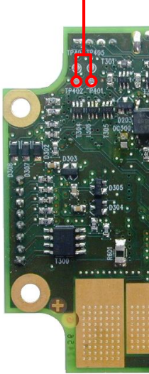
Figure 5.1 Reset to factory default settings
