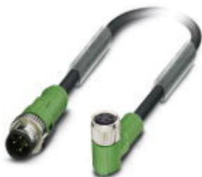
Sensor/actuator cable, 4-position, Variable cable type, Plug straight M12 SPEEDCON, A-coded, on Socket angled M8, cable length: Free input (0.2 ... 40.0 m)
