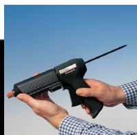
Push Heating Head onto Handle
